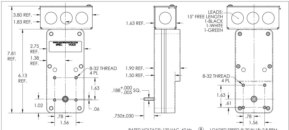
RATED VOLTAGE: 120 VAC, 60 Hz ROTATION: CW NO LOAD SPEED: 2.9 RPM
