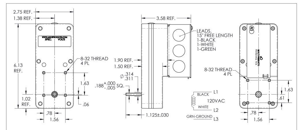
RATED VOLTAGE: 120 VAC, 60 Hz ROTATION: CW
