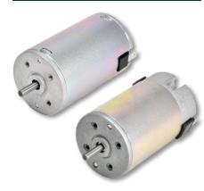
The 28Y DC is a medium frame, precision PMDC motor with various speed options. Featuring permanent neodymium magnets and copper brushes. The 28Y can be fitted to a variety of Multi's standard, compact, and planetary gearbox options. Speed is rated from 2540 to 5615 RPM at max efficiency. Bi-directional. Optional encoders and other accessories. Designed for continuous or intermittent duty.
