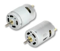
The 315 DC is the smallest frame economical PMDC motor option. Featuring permanent ferrite magnets and carbon brushes that can be fitted to a variety of Multi's gearboxes and reducer options. Speeds from 2900 up to 11600 RPM, Bi-directional. Optional EMI filtering and other accessories. Designed for continuous or intermittent duty.
