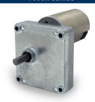
The 7000x Series "Square" features the same variety of industry standard mounting options as the 7000 series but with an offset output shaft. Able to handle a continuous torque rating up to 75 in-lb. Output shaft diameters range from 1/4" through 3/8" with dual outputs, flats, keyways, threads, or square ends. Other options: multiple gearing materials, needle or ball bearings, and custom wiring harnesses.
