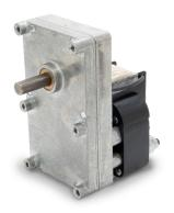
The 9000 Series is the largest and most robust gearbox we offer. Capable of handling torque ratings up to 200 in-lb continuously or up to 300 in-lb intermittently. Constructed with a zinc die-cast housing. Output shaft diameters range from 1/4" through 3/8" with flats, keyways, threads, square ends, or hollow-thru shafts. Other options: multiple gearing materials, needle or ball bearings, and custom wiring harnesses.
