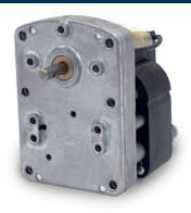
The 6000 Series offers industry standard mountings on both sides of the housing. Able to handle a continuous torque rating up to 75 in-lb. Low speed output of 8- 25 RPM. Output shaft diameters range from 1/4" through 3/8" with flats, keyways, threads, or square ends to meet your application needs. Other options: multiple gearing materials, needle or ball bearings, and custom wiring harnesses.
