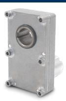
The 9000 Series is the largest and most robust gearbox we offer. Capable of handling torque ratings up to 200 in-lb continuously or up to 300 in-lb intermittently. Constructed with a zinc die-cast housing. Output shaft diameters range from 1/4" through 3/8" with flats, keyways, threads, square ends, or hollow-thru shafts. Other options: multiple gearing materials, needle or ball bearings, and custom wiring harnesses.
