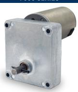
The 7000 Series "Square" features several available casting covers with a variety of industry standard mounting options to fit any application. Able to handle a continuous torque rating up to 75 in-lb. Output shaft diameters range from 1/4" through 3/8" with dual outputs, flats, keyways, threads, or square ends. Other options: multiple gearing materials, needle or ball bearings, and custom wiring harnesses.
