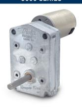
The 3000 Series is our newest gearcase design, offering industry standard mountings on both sides of the housing. Able to handle a continuous torque rating up to 75 in-lb. Output shaft diameters range from 1/4" through 3/8" with dual outputs, flats, keyways, threads, or square ends to meet your application needs. Other options: multiple gearing materials, needle or ball bearings, and custom wiring harnesses.
