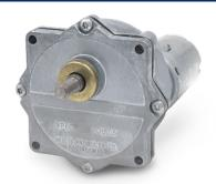
The heavy-duty 302 Series "Star" shaped gearbox offers a compact footprint for when surface area is at a premium. The 302 gearcase can handle a continuous torque rating up to 150 inlb. Constructed with a zinc die-cast, gasket-sealed housing for dust and moisture resistance. Output shaft diameters range from 1/4" through 3/8" with flats, keyways, threads, or square ends to meet your application needs. Other options: multiple gearing materials, needle or ball bearings, and custom wiring harnesses.
