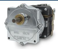
The heavy-duty 302 Series "Star" shaped gearbox offers a compact footprint for when surface area is at a premium. Able to handle a continuous torque rating up to 150 in-lb. Constructed with a zinc die-cast, gasket-sealed housing for dust and moisture resistance. Output shaft diameters range from 1/4" through 3/8" with flats, keyways, threads, or square ends to meet your application needs. Other options: multiple gearing materials, needle or ball bearings, and custom wiring harnesses.
