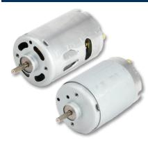
The 615 DC is a medium frame economical PMDC motor option. Featuring permanent ferrite magnets and carbon brushes that can be fitted to a variety of Multi's gearboxes and reducer options. Optional EMI filtering and other accessories.
