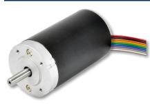
The Digital Drive Brushless DC from Multi Products is the most controllable motor in our line. Compact, powerful, and precise. Featuring a 6 pole stator and slotless rotor design for high torque density. The motor utilizes an integral motor drive system capable of using digital input / output signals from external sensors to control the speed, torque, and position of the motor. Optional encoders and other accessories. Designed for continuous or intermittent duty.
