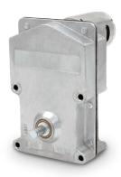
The rugged 1600 Series is designed for tough applications. Able to handle a continuous torque rating up to 150 in-lb. Constructed with a zinc die-cast, gasket-sealed housing for dust and moisture resistance. Output shaft diameters range from 1/4" through 3/8" with flats, keyways, threads, or square ends to meet your application needs. An optional dust cover over the motor is available.
