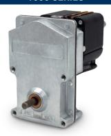
The rugged 1600 Series is designed for tough applications. Able to handle a continuous torque rating up to 150 in-lb. Constructed with a zinc die-cast, gasket-sealed housing for dust and moisture resistance. Output shaft diameters range from 3/8" through 1/2" with dual outputs, flats, keyways, threads, or square ends to meet your application needs. An optional dust cover over the motor.
