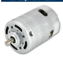
The 983 DC is the largest frame economical PMDC motor option. Featuring permanent ferrite magnets and carbon brushes that can be fitted to a variety of Multi's gearboxes and reducer options. Speeds from 3100 and 4800 RPM Bi-directional. Optional EMI filtering and other accessories. Best for high starting torque, intermittent duty applications.
