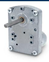
The 6000 Series offers industry standard mountings on both sides of the housing. Able to handle a continuous torque rating up to 75 in-lb. Low speed output of 8- 25 RPM. Output shaft diameters range from 1/4" through 3/8" with dual outputs, flats, keyways, threads, or square ends to meet your application needs. Other options: multiple gearing materials, needle or ball bearings, and custom wiring harnesses.
