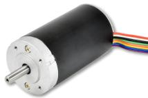
The Hall Effect Brushless DC from Multi Products is compact, powerful, and precise. Featuring a 6 pole stator and slotless rotor design for high torque density. The Hall Effect BLDC motor is designed to connect to an external drive system utilizing the 3 onboard Hall Effect sensors for control and positioning. Reversible. Optional encoders and other accessories. Designed for continuous or intermittent duty.
