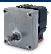
The 7000 Series "Square" features several available casting covers with a variety of industry standard mounting options to fit any application. Able to handle a continuous torque rating up to 75 in-lb. Output shaft diameters range from 1/4" through 3/8" with flats, keyways, threads, or square ends. Other options: multiple gearing materials, needle or ball bearings, and custom wiring harnesses.
