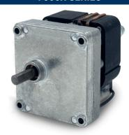
The 7000x Series "Square" features the same variety of industry standard mounting options as the 7000 series but with an offset output shaft, allowing for greater gearing reduction and lower output speeds. Able to handle a continuous torque rating up to 75 in-lb. Output shaft diameters range from 1/4" through 3/8" with flats, keyways, threads, or square ends. Other options: multiple gearing materials, needle or ball bearings, and custom wiring harnesses.
