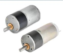
The GBS35 / GBM35 is an economical 35 mm offset in-line shaft gearbox suitable for lower torque applications. Compact, quiet and versatile with a continuous torque rating up to 10 in.-lbs. Great for low-torque intermittent duty applications such as gaming and office equipment. Different mounting patterns and output shaft diameters distinguish the GBS and GBM from each other. GBS35 features cut steel gearing, whereas the GBM35 features sintered steel gearing.
