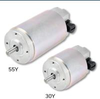
The 30Y & 55Y DCs are the largest frame precision PMDC motor options. Featuring permanent neodymium magnets and copper brush commutation. They can be fitted to a variey of Multi's standard, compact, and planetary gearbox options. Speed is rated from 1275 to 4700 RPM. Bi-directional. Optional encoders and other accessories available. Designed for continuous or intermittent duty.
