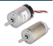
The 12Y & 18Y DCs are the smallest frame precision PMDC motor option. Featuring permanent neodymium magnets and copper or silver graphite brushes. The 18Y can be fitted to a variety of Multi's standard, compact, and planetary gearbox options. Speed is rated from 2685 - 5570 RPM at max efficiency. Bi-directional. Optional encoders and other accessories. Designed for continuous or intermittent duty.
