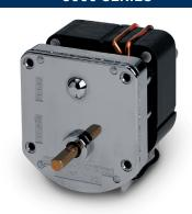
The 8000 Series "D" is the smallest gearbox we offer, with an industry standard mounting option for the ability to easily retrofit into existing light-duty food service, gaming, and vending applications. Able to handle a continuous torque rating up to 50 in-lb. Output shaft diameters range from 1/4" through 3/8" with flats, keyways, threads, or square ends. Other options: multiple gearing materials, needle or ball bearings, and custom wiring harnesses.
